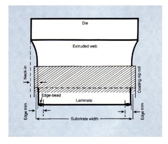
Neck-in can arise as a result of surface tension as the polymer leaves the die, as well as due to melt elasticity effects that occur during the process. The problem with neck-in is that it significantly reduces the amount of substrate that can be covered with the coating. Any reduction in width as the polymer leaves the die will leave areas of the substrate without a coating. The area that isn't covered is unusable and will need to be discarded, leading to a significant amount of waste.
